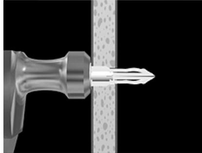
Photo D - Insert anchor in hole and tap flush with wall.
