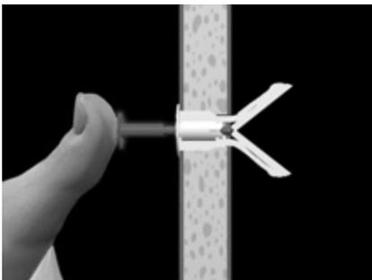
Photo E - Insert key to pop anchor open & lock behind hollow wall (not necessary for thick or solid walls). Do not force or hammer key.
