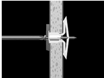
Photo F - Place item over anchor. Insert screw and tighten until screw is flush with fixture. Then, stop. The anchors also wedge securely in thick or solid walls, or in wood studs behind drywall.
